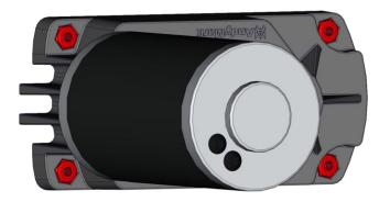
**Step 8**: Insert a Motor Assembly into the open hole, and secure it with two 10-32 x 0.625 in. Socket Head Cap Screws with Nylon Thread Lock Patch (am-1120).
