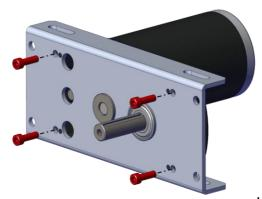
**Step 11:** Run the motor for several minutes to break in the gear pairs. Remove the Toughbox Micro from the plate, grease all gears, and reattach the gearbox to its' plate.
